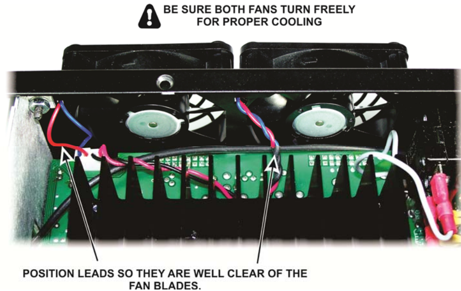
Figure 11. Positioning the Fan Leads.
